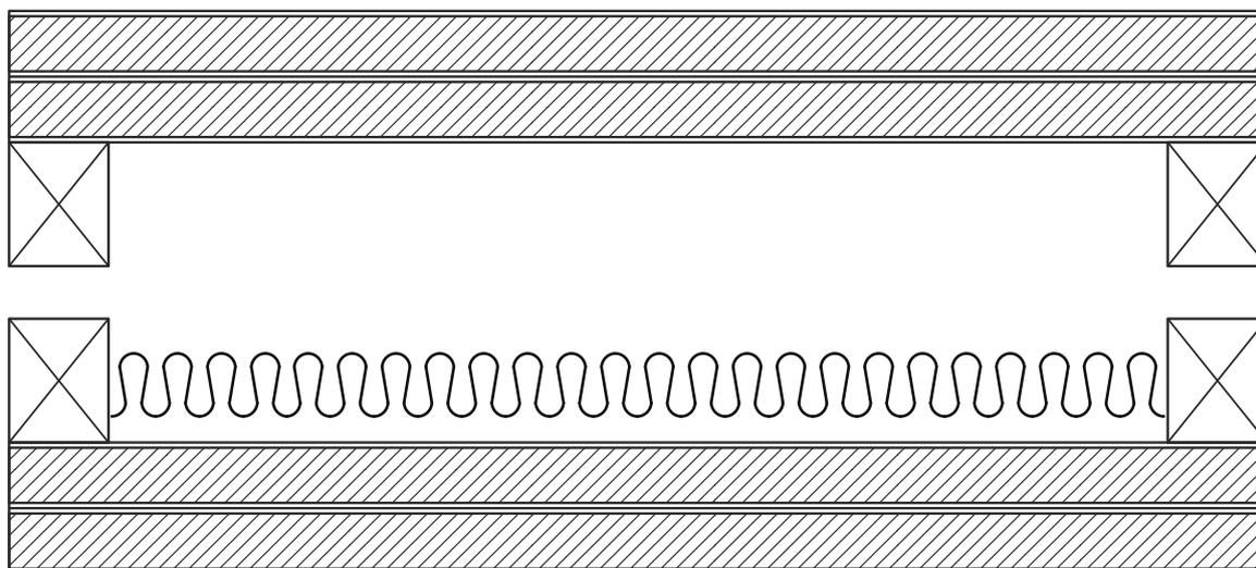
**Figure S28C7b: One row of 70 mm x 35 mm staggered timber studs without noggings between adjacent studs**
