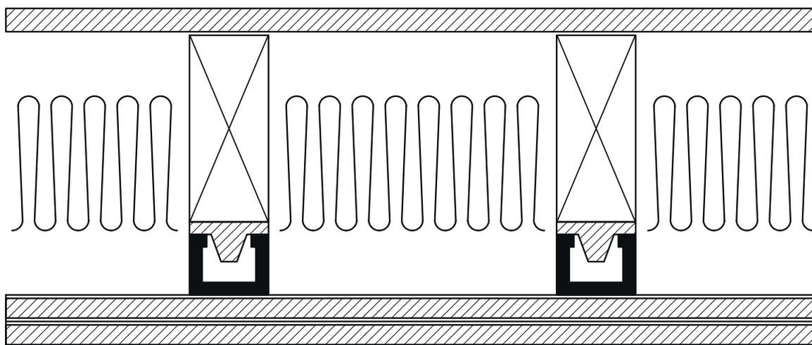
Figure S28C10b: Timber flooring with minimum 8.5kg/m<sup>2</sup> mass, over 19 mm thick particleboard floor sheeting
