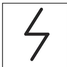
Figure S23C7d: End-of-line device symbol
