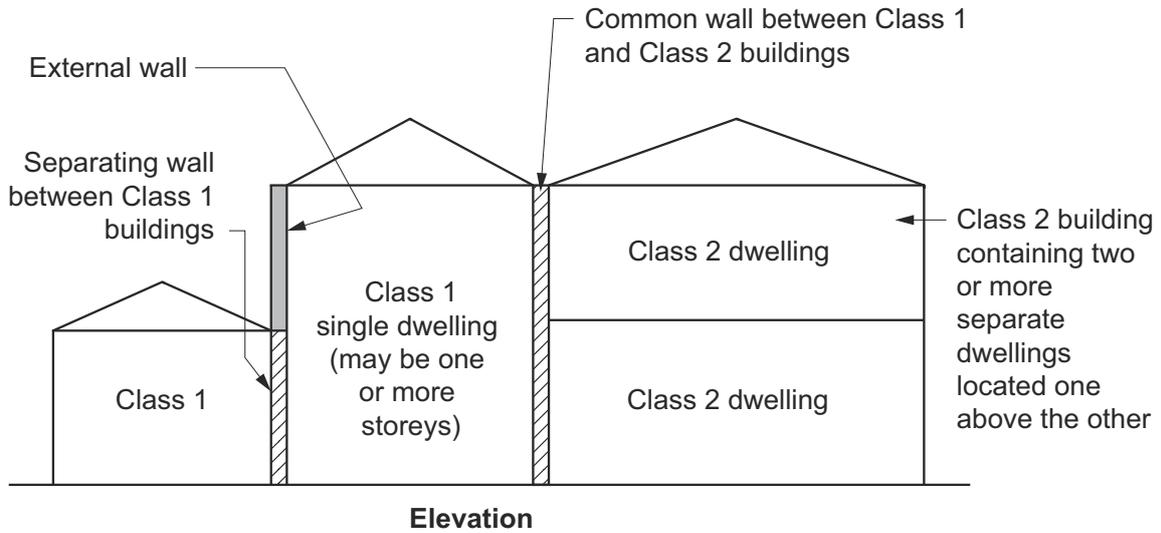
Figure A6G2b: Typical Class 1 building configurations
