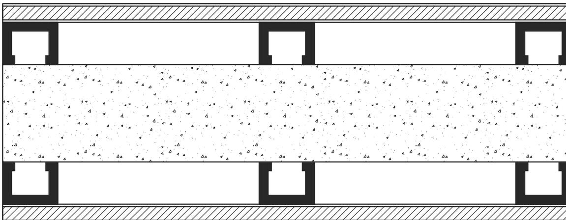
Figure S28C5c: 200 mm thick concrete panel with one layer of 13 mm plasterboard or 13 mm cement render on each face
