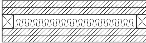
Figure S28C7d: One row of 70 mm x 35 mm timber studs at not less than 450 mm centres
