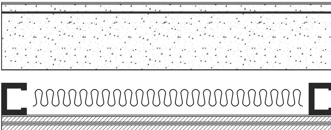
Figure S28C5e: 125 mm thick concrete panel with studs, insulation and plasterboard
