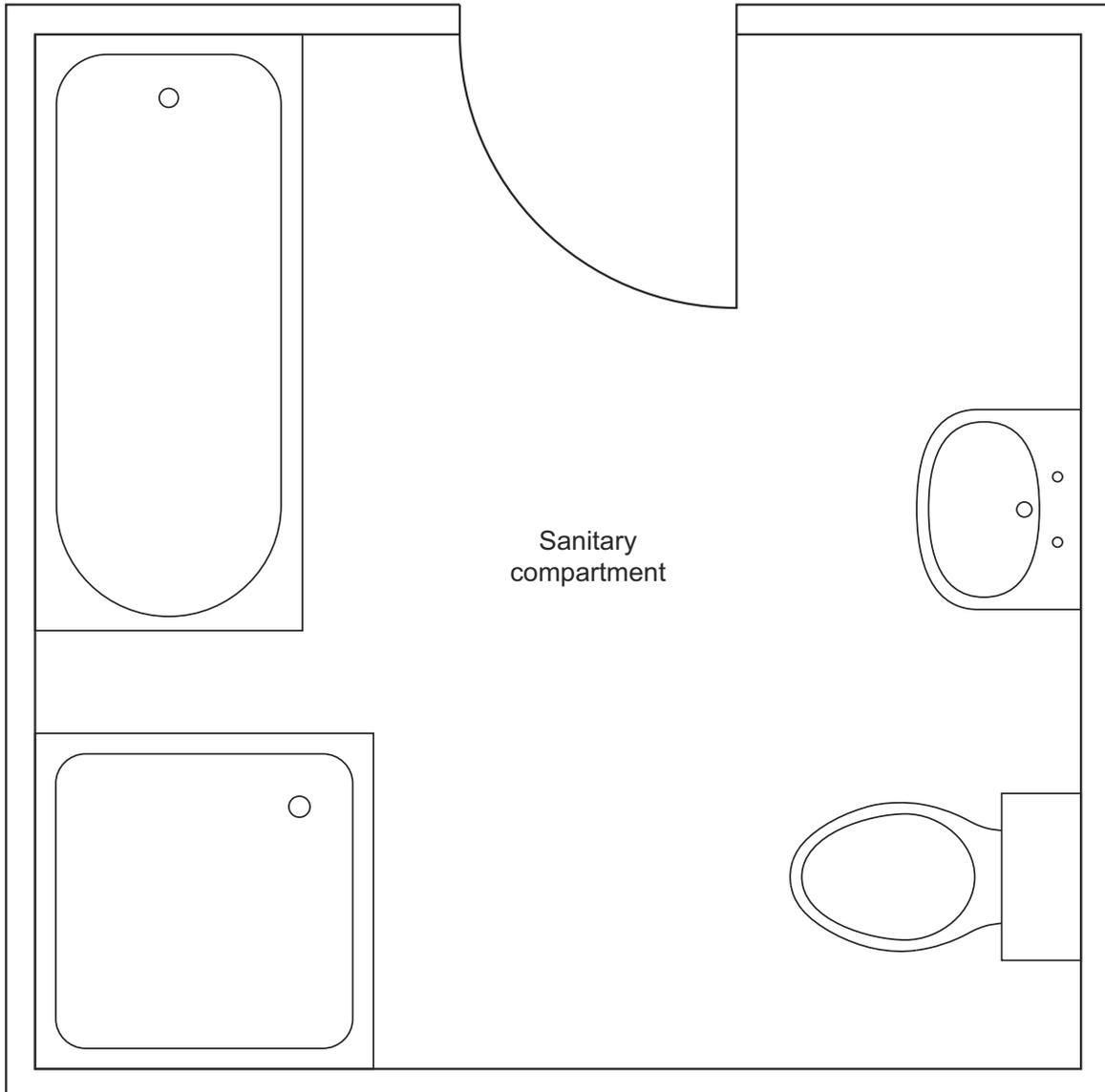
**Figure 6b: Identification of a sanitary compartment (diagram b)**
