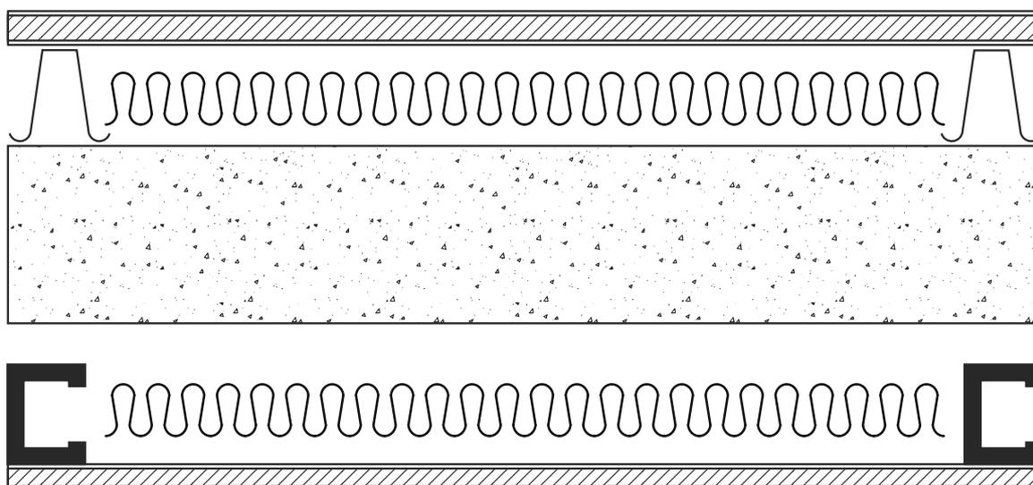
Figure S28C6c: Two leaves of 75 mm autoclaved aerated concrete wall panel
