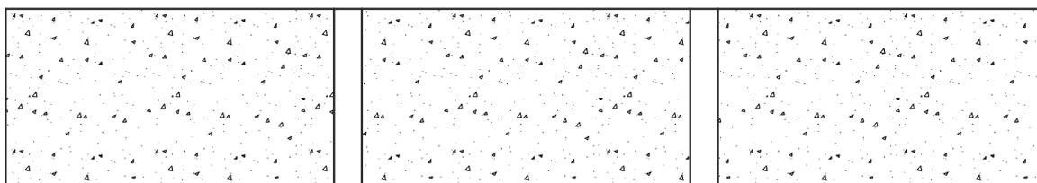
Figure S28C5i: 140 mm thick concrete blockwork with timber battens and 13 mm plasterboard
