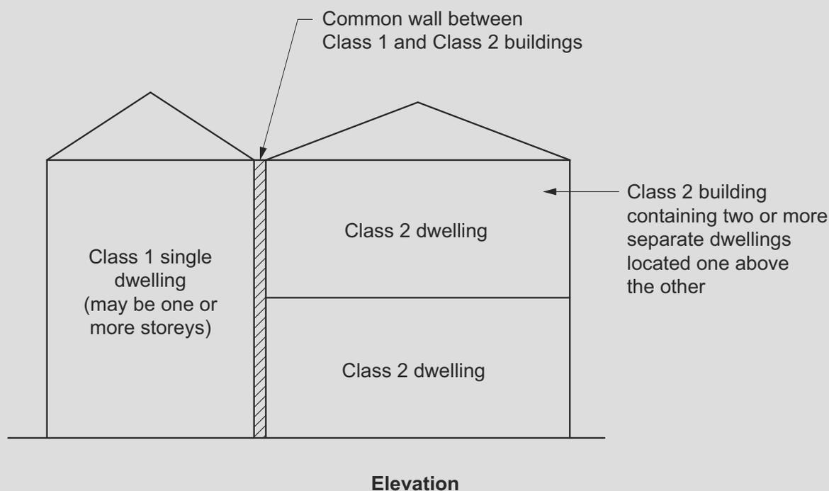
Figure A6G3b (explanatory): Elevation showing a single storey of Class 2 with a common area below
