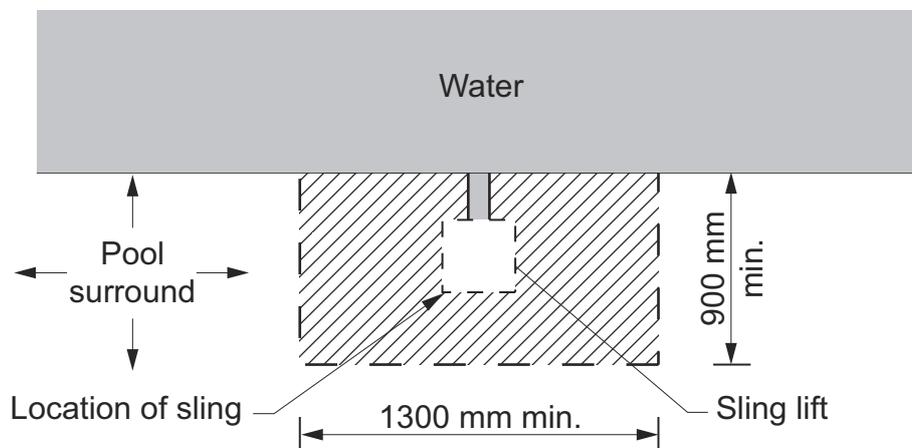
Figure S16C5b: Clear swimming pool surround space for sling lift in the transfer position — Sectional elevation
