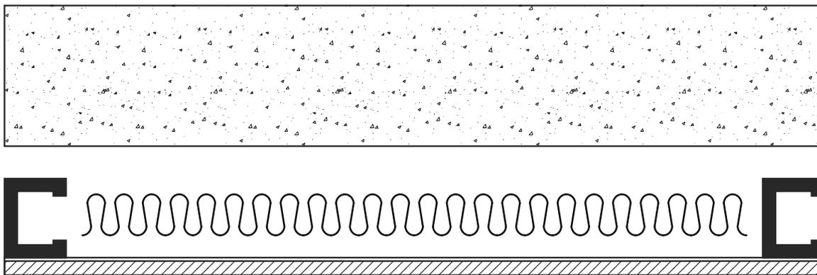
Figure S28C5f: 125 mm thick concrete panel
