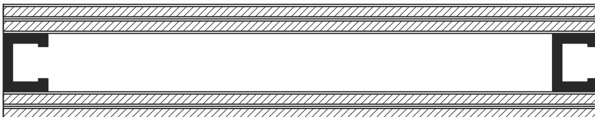
Figure S28C7i: One row of 64 mm steel studs
