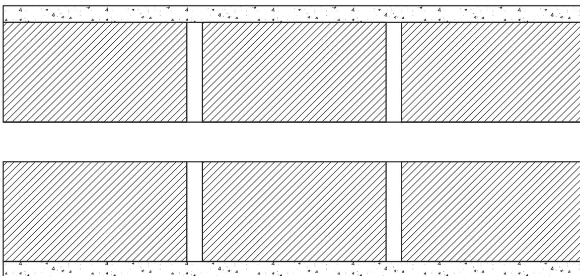
Figure S28C4c: Single leaf of 110 mm clay brick masonry
