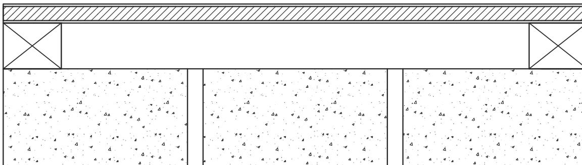
Figure S28C5j: 100 mm thick concrete panel
