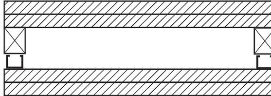
Figure S28C7e: Two rows of 64 mm steel studs at 600 mm centres (Method 1)
