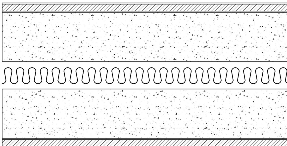
Figure S28C6d: 75 mm thick autoclaved aerated concrete wall panel (method 3)
