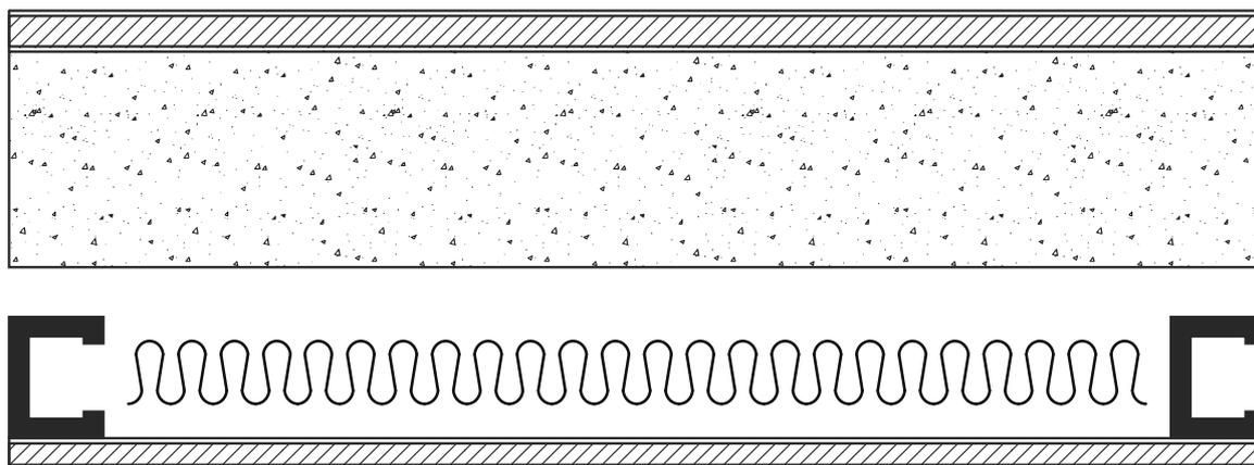
Figure S28C6b: 75 mm thick autoclaved aerated concrete wall panel (method 2)
