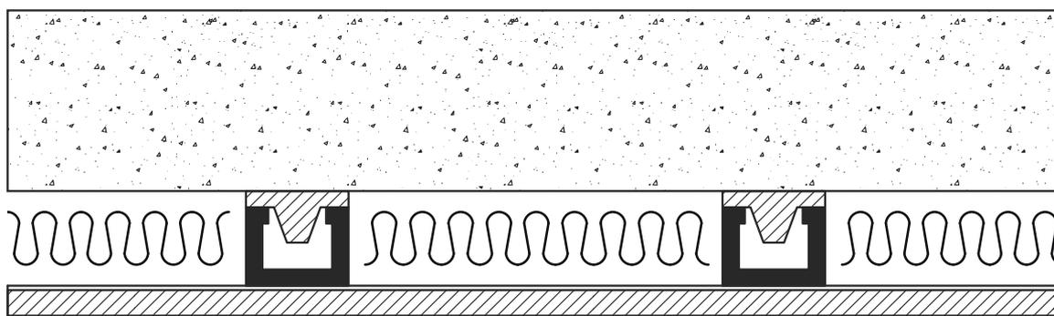
Figure S28C8b: 200 mm thick concrete slab with carpet on underlay
