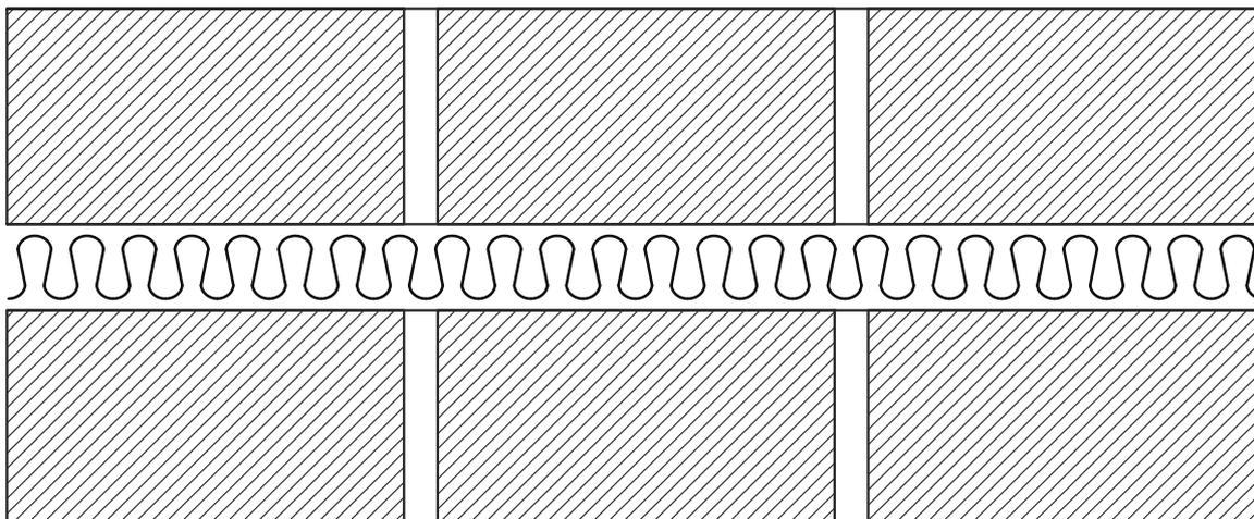
Figure S28C4b: Two leaves of 110 mm clay brick masonry (method 2)
