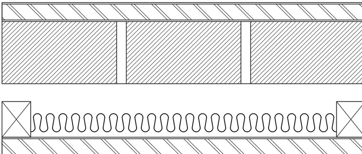
Figure S28C4d: Single leaf of 90 mm clay brick masonry
