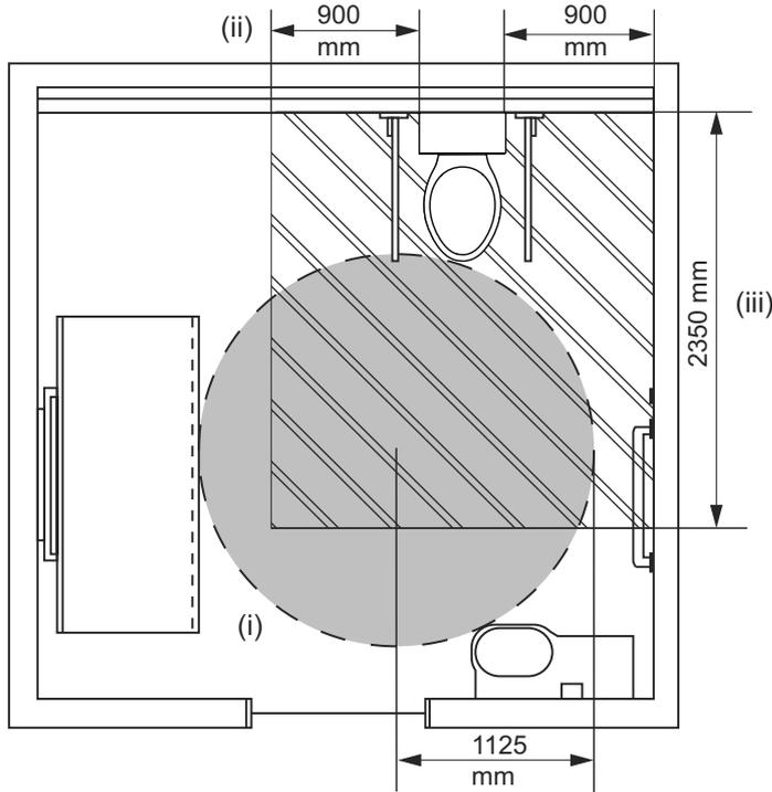
Figure S27C2b: Required circulation spaces — Turning space and circulation space for a washbasin
