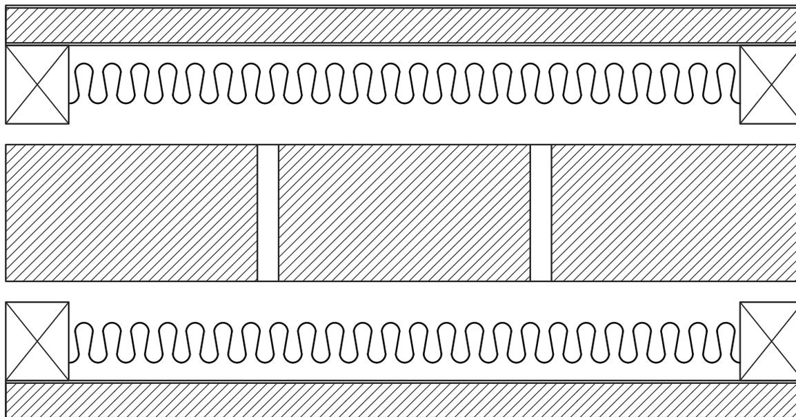
Figure S28C4e: Single leaf of 150 mm brick masonry with 13 mm cement render on each face
