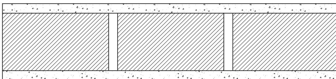
Figure S28C4h: 110 mm thick concrete brickwork
